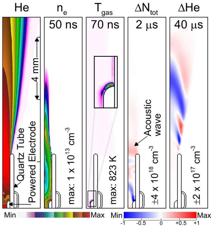
In this paper, the results from a 2-dimensional plasma hydrodynamics model of an APPJ are discussed. The device modeled consists of helium flowing through a 1 mm diameter quartz tube, with an annular high voltage electrode inside the tube, shown at the left. The plasma propagates in tens of ns as an ionization wave beginning at the powered electrode, producing the electron densities shown in the figure ( $n_e$ ).
